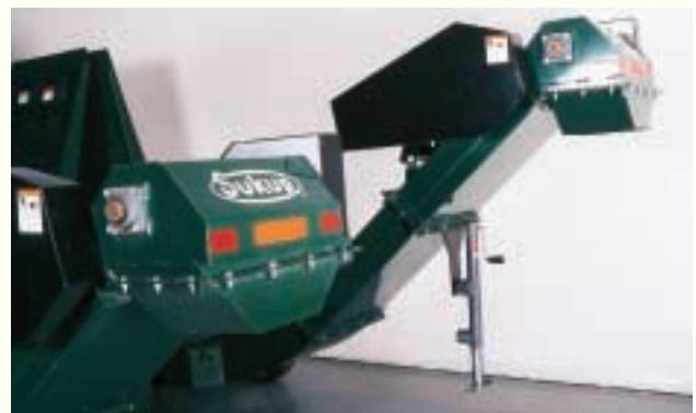
Standard spout shown in foreground, Spout with optional extension at back.
